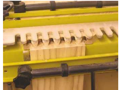
▲ Pic.5 An inexpensive routing jig produces dovetails to the same pitch as on Ercol production furniture
